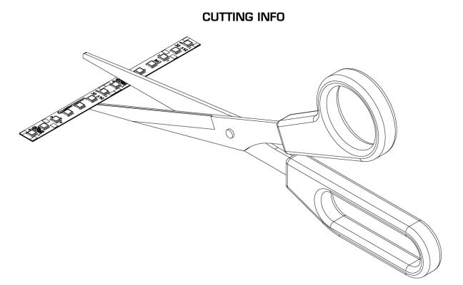
The LED strip can be separated or shortened every 50 mm. On the back of the LED strip is a double-sided heat-conducting adhesive tape, which allows installation of the LED strip. Professional LED strips can be cut with scissors.
